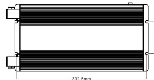
BLP-1000S-12V-*/BLP-1000S-24V-* Inverter installation size
